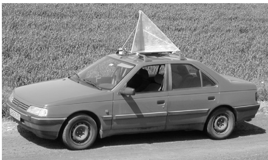
Figure 2: A standard civilian car with a corner reflector on the roof used as a moving target.
